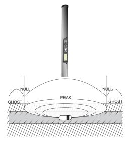
Start by following the suspected path of the pipe. Stop locating when the PEAK reading is found. Then rotate the **Receiver** as shown in the figure below. When pivoting the **Receiver**, do not change the vertical position. The **Receiver** will indicate a peak when the **Receiver** antenna is in line with the Sonde.
