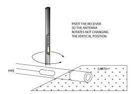
Now move the **RECEIVER** side to side (across the path of the pipe) as shown below. When the PEAK is found, the **RECEIVER** is directly over the Sonde. Mark this location. Next, check for ghost signals in front of and in back of the Sonde to confirm the location.
