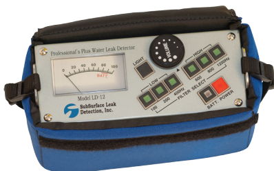
AMPLIFIER WITH METER DISPLAY AND FILTER CONTROLS
