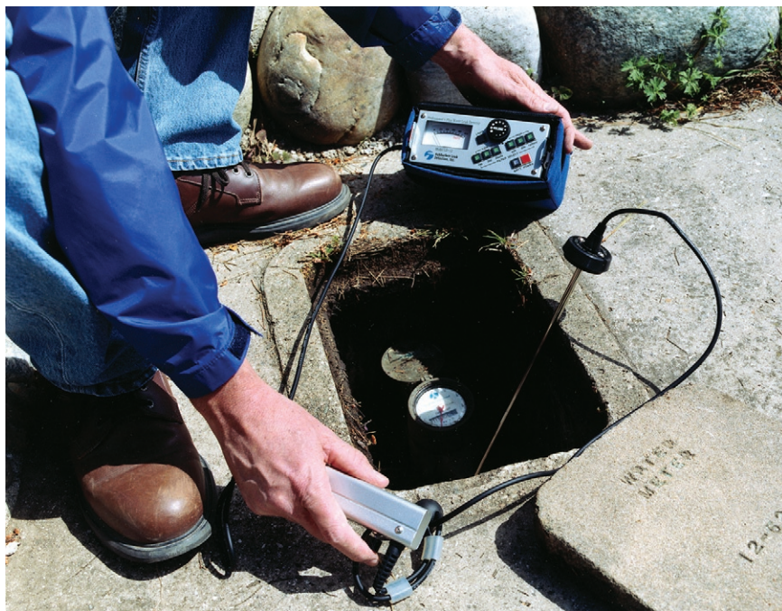
Figure 4-8 Leak Survey at a Meter
