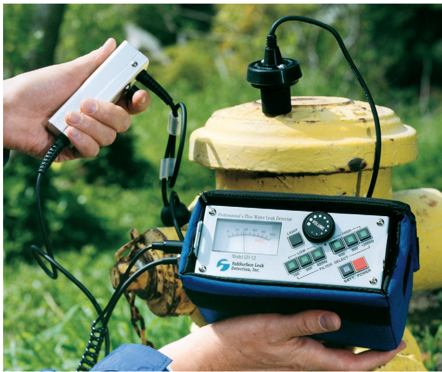
Figure 4-6 Leak Survey at a Hydrant
