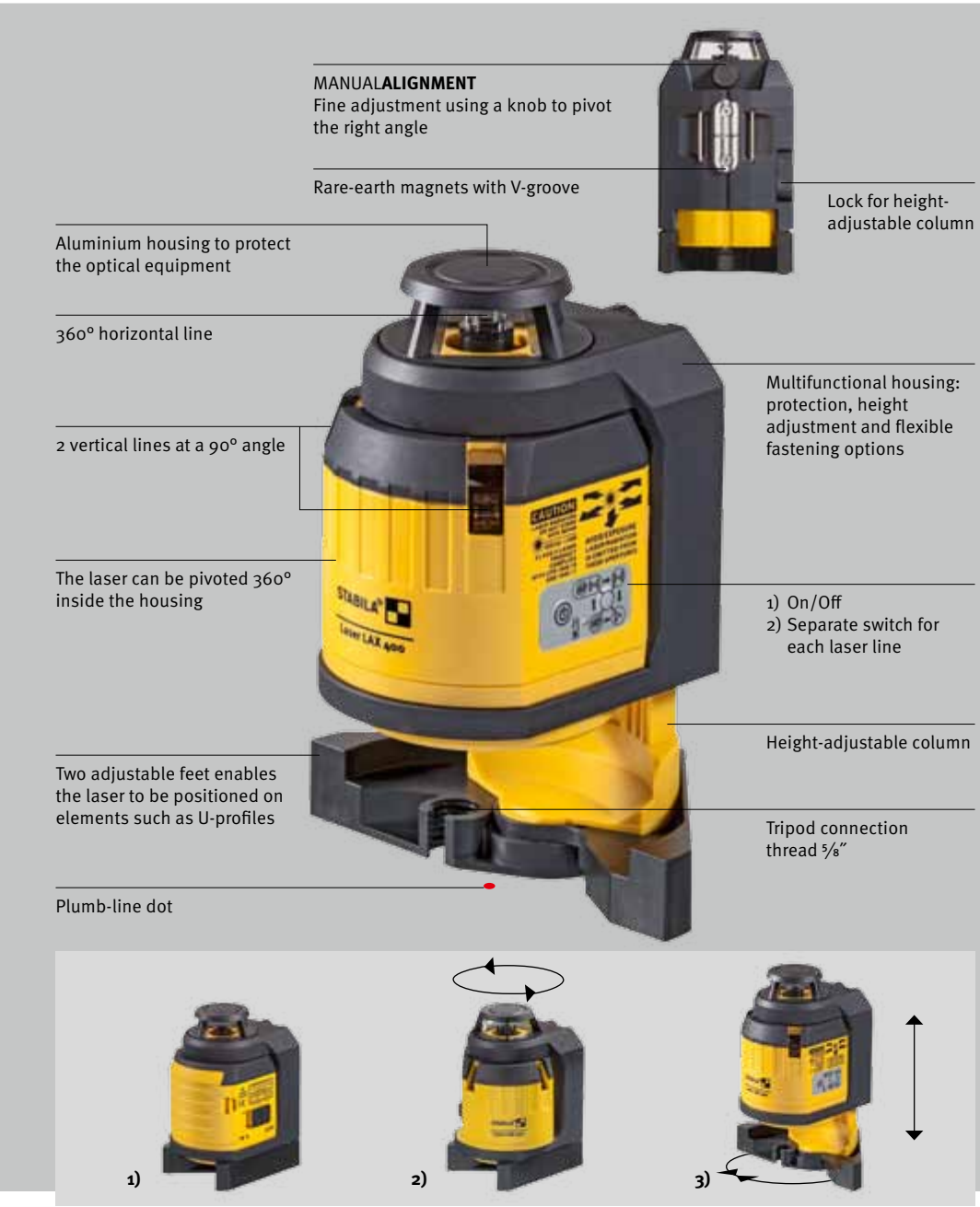
1) Park position. 2) Housing can pivot 360° inside the U-shaped housing. 3) The height of the laser can be adjusted thanks to the extendable column. The two adjustable feet enables the laser to be positioned on elements such as U-profiles.
