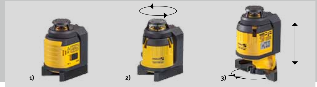
1) Park position. 2) Housing can pivot 360° inside the U-shaped housing. 3) The height of the laser can be adjusted thanks to the extendable column. The two adjustable feet enables the laser to be positioned on elements such as U-profiles.
