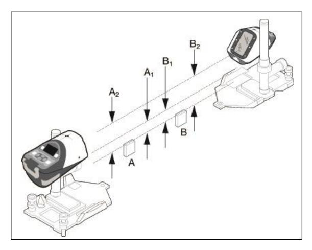
Checking the calibration of your pipe laser is easy. All you need is an engineer's rule and your pipe laser.
