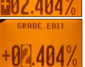
**Automatic Spot Align (only DG813)** - The Spot Finder SF803 guides the beam to the target point in the horizontal axis, while the Z-axis grade value will be maintained.
