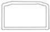
Rectangular shape allows for laser detectors to be mounted directly to the rod - no bracket required!
