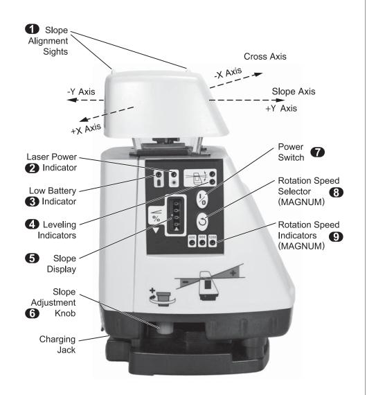
Note: Controls and displays are the same for both models except that the AS2 MAGNUM has a rotation speed selection button speed indicator LEDs and the S2 Compound slope adapter on top of the slope alignment sights.
