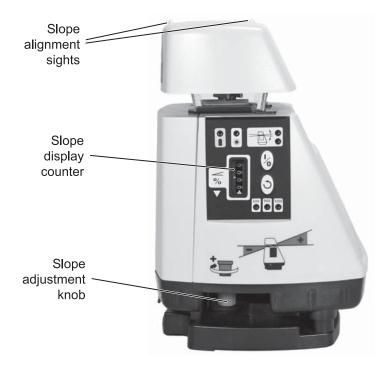
**Note:** When using either AS2 model at slope settings over 14%, you will need to tilt the tripod to allow the laser to reach the desired slope. By aligning the laser so that one tripod leg is to the rear (down slope side), you can shorten that leg to tilt the tripod head and the setup will remain stable.
