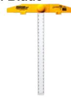
Perforated (1/16" offset) 24" blade accepts utility knife point for fast, efficient drywall scoring, Molded high impact head with hand grip and board guide, Screened, thermal-bonded black 1/8" 1/16" or mm (metric) graduations, Large, bold graduations are easy reading, Extruded aluminum blade assures durability
