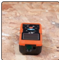
Cal3: Rotate 180°, LCD towards you.
