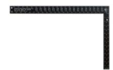
24" x 2" body, 16" x 1-1/2" tongue, 1/8" thick, Aluminum body will not rust, Laser etched EZ Read graduations and numbers on black anodized body, Graduations measure 1/8", 1/10", 1/12", 1/16", Includes octagon scales, rafter tables, brace tables and board foot tables.
