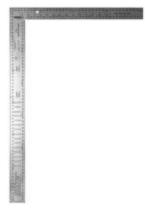
600mm x 50mm body, 400mm x 38mm tongue, 3mm thick, EZ Read™ thermal bonded numbers and graduations, Graduations measure in 2mm increments, Metric rafter conversion tables
