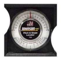
High-Impact molded body, Easy-to-read increments from 0-90 degrees printed on durable acrylic lens, Printed scale reads pitch in inch rise per 12" run without conversion tables
