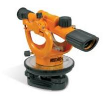
Horizontal circle - graduated to single degrees and reads by vernier direct to 15 minutes, Vertical arc - reads to degrees 45-0-45, Horizontal tangent screw and vertical lock and tangent screw for precise movement control, Top mounted leveling vial - for effortless viewing, Large leveling screws - easy to turn, 40-6910 Includes > Builder's transit level, instruction manual with warranty card, hard-shell carrying case
