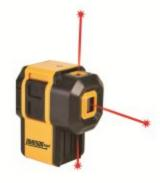
Projects 2 plumb dots and 1 level dot. Tall profile for clearance of wood or metal drywall track. Locking compensator protects pendulum during transport. Visual out-of-level indicator. 1/4" tripod thread for use with most common tripods. Dust resistant construction. 40-6646 INCLUDES > Laser, 2 "AA" alkaline batteries.
