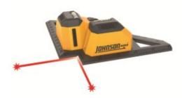
Laser beams project over wet mastic or concrete. Perpendicular lasers form a 90° reference for flooring installation. Dual leveling vials for use on vertical surfaces. Ruled ends - inch, metric, and angle. 40-6624 INCLUDES > Laser, 2 "AA" alkaline batteries.
