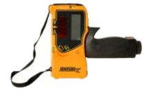
With this laser detector, a line generated pulse laser level can be used both indoors with bright light and/or outdoors in the sunlight where the beams are not visible, Audible and visual indicators for precise leveling, Clamp attaches to grade rods, Use with 40-6602 & 40-6662 line-generating lasers with pulse, 40-6780 Includes > Detector, 9V battery, clamp
