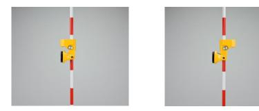
Prism canister can be switch to either way. This is very handy for surveying corner point.
