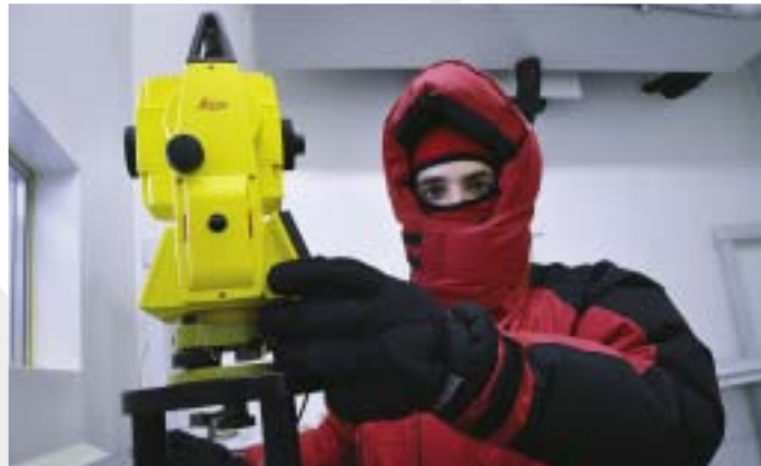
Performance check at -30°C in an accessible climatic chamber
