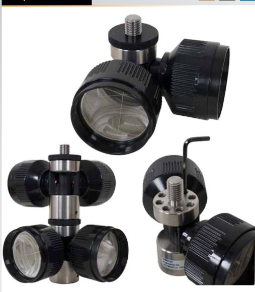
**PART NO** DESCRIPTION 6603-03 62 mm Adjustable Dual Prism, 0 offset, 5/8 x 11 compatible 6603-03-050 Holder only, compatible with all M20 X2 screw in prisms 6603-00-005-TMB
