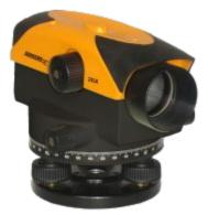
Water and dust resistant, Wire-hung, magnetically dampened compensator, Large, easy-to-use focusing knob and fine adjusent knobs on left and right sides with endless horizontal drive, 360 degrees horizontal circle, Prism for bubble viewing and a top-mounted optical sight for quick reference, 1:100 stadia for distance estimation, Includes > Automatic level, instruction manual with warranty card, hard-shell carrying case
