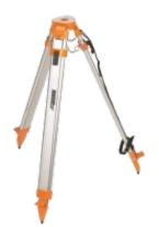
Durable aluminum construction with extendable legs, Adjustment range 3 ft. 3in. to 5 ft. 3 in. (nominal length), Quick connection for lasers with 5/8" - 11 threads, Quick clamp lock offers quick and secure clamping, Feet have sharp metal points for use on uneven outdoor terrain and removable rubber covers for use indoors, Safety chains prevent legs from accidental collapse, Carrying strap included
