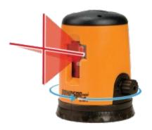
Self-leveling within +/-6 degrees, Interior horizontal and vertical layout, Locking mechanism protects inner pendulum during transportation, 360 degrees graduated base allows angle layout, Emits cross line lasers, Projects vertical and horizontal laser lines simultaneously, Visual out of level indicator, 5/8" - 11 thread, 40-0912 Includes > Laser, 3 "AAA" alkaline batteries, instruction manual with warranty card, soft-sided carrying case
